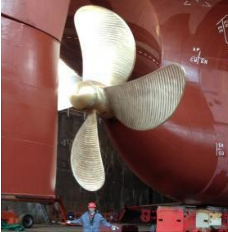
1- Sabit Kanatlı Pervane (FP) Fixed propeller,
