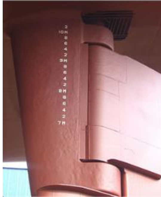
Rudder hanging Castings.
