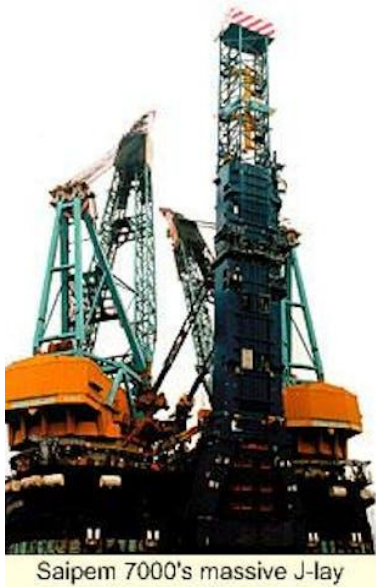
“Saipem 7000” Cranes: 2 x 7000 Tons. 140 m.long Boom
