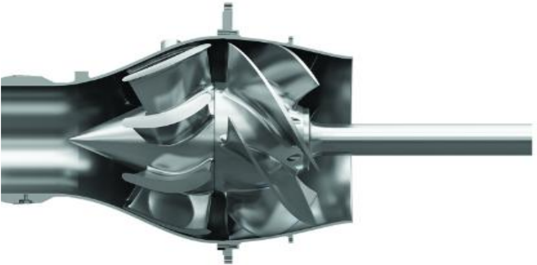
SS Water Jet Propulsion system.
