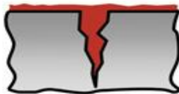
3 Application of penetrant
