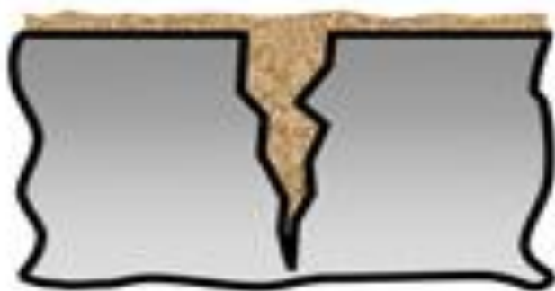
1 Crack filled with dirt
