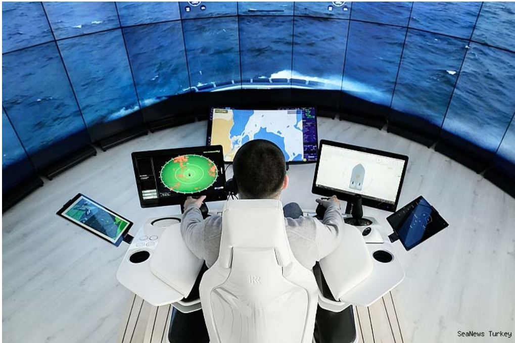
Photo-1: Remote-Captain of the tug operating the tug Svitzer Hermod at Remote Operation Centre. (Photo: SeaNews Turkey- www.seanews.com.tr )
