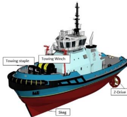
Figure 1. An escort tug with ASD thrusters.
